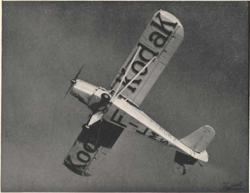
Another Auster used for aerial photography is shown in this unusual view. Owned by M. Ray Delvert of Paris, a professional photographer, M. Delvert has modified his aircraft by cutting down the Port cabin door to provide increased vertical deflection for his large hand held camera.
