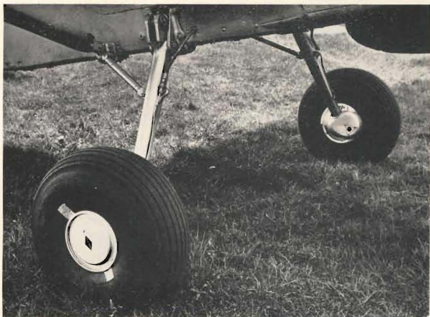
A new feature of the Mk. 9 is the sturdy liquid-sprung undercarriage. Low pressure tyres of 1 ft. 9 in. dia. are fitted together with Goodyear single disc type brakes.
