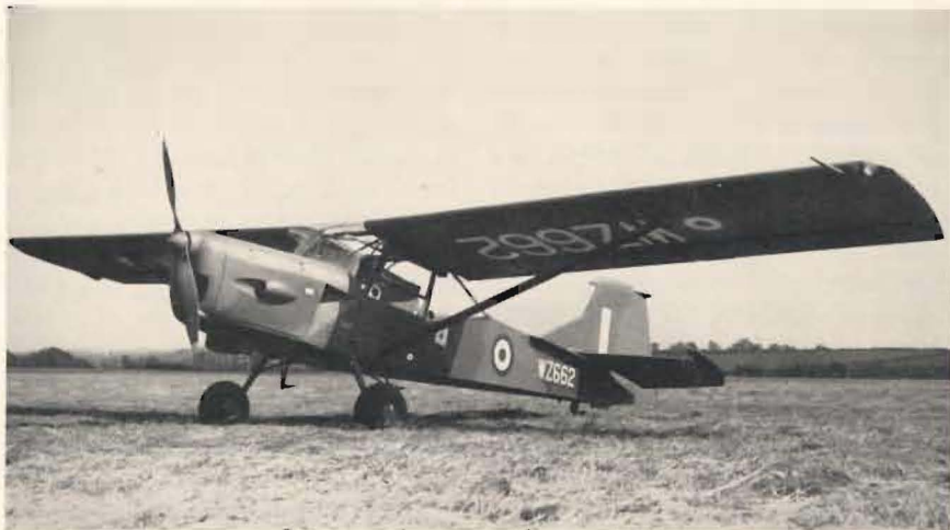
This view clearly shows the difference between the new Mk. 9 and previous military Austers, namely, the single lift strut, a cleaner wing with split flaps, bigger tyres and cantilever tail surfaces.
